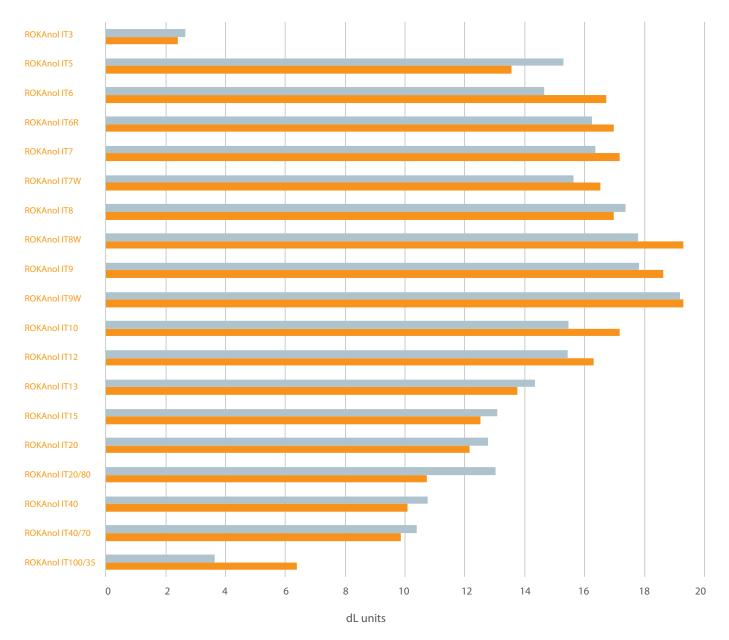
The dL parameter is described by perceptually uniform, trichromatic colour models: CIE LAB and CIE LCH. The following is an interpretation of this parameter: L is defined as lightness (luminosity), while dL is determined by the equation: dL = LT - LS, where: T – tested sample (fabric after the detergency test), S – standard to which the tested sample is compared (fabric before the detergency test).
