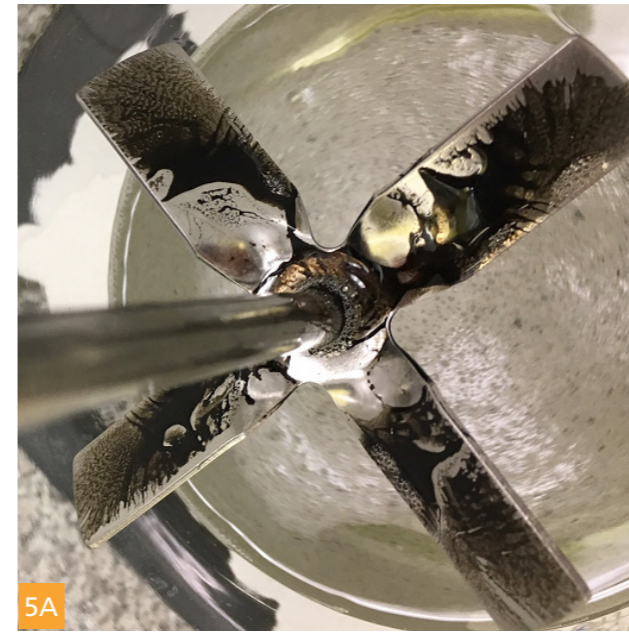
Pic. 5A/5B Degreasing capability. Dynamic test, ROKANOL GA8, after 2 min and 5 min
