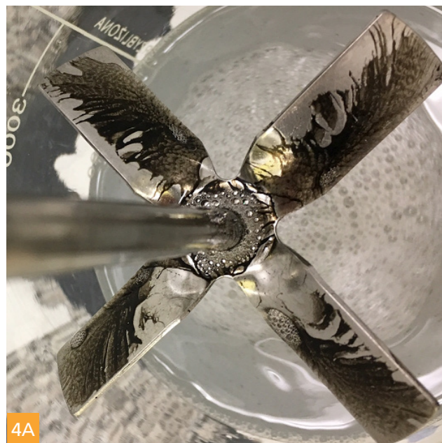
Pic. 4A/4B Degreasing capability. Dynamic test, ROKANOL GA7, after 2 min and 5 min
