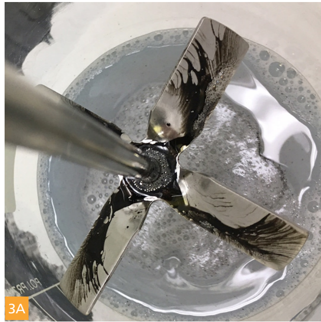
Pic. 3A/3B Degreasing capability. Dynamic test, ROKANOL GA5, after 2 min and 5 min
